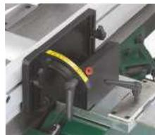
**Sturdy Fence System** The fence can tilt up to 45° and is supported by a strong mounting system.
